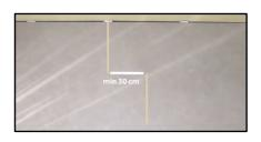
Always ensure that the ends of the tiles in two successive rows are the same and that the distance between the short ends is at least 30 cm.
