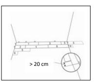
Always ensure that the ends of the tiles in two successive rows are the same and that the distance between the short ends is at least 20 cm.
