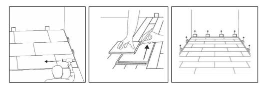
1. For the installation of the last row, you will have to saw the boards lengthwise. You can use a metal striking bar to insert the boards into the click system of the previous row. Please note: hitting the boards too hard or too unevenly can damage the boards and their click connections.
